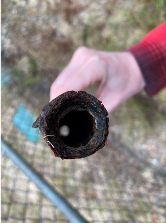
Figure 6: Photo of a Corroded Pipe Found at the Eulonia, Georgia, Site
